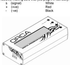
Connect the battery wires to a charged pack of battery. Turn on the ESC and the setting card will activate automatically. Note that the screen will show "Loading ... " during initialization - indicating that the ESC is copying the current setup in the ESC to the setting card. Once loading is completed, the screen will show "ORCA VRITRA-VTC - Program". You can now start to program your ESC.
